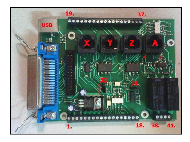
The HDBB breakout board was designed to use with our Whale2(-T)\*, Whale3, Mammut\* and Dugong servo drives or with any other third party stepper or servo drives which using step and direction control signals.
